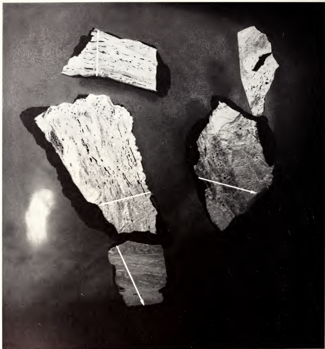
FIG. 17.—34.11. Fragments of remnant oxide from metal blade of dagger axe, mounted in plastic and polished for microscopic and electron microprobe examination; \times 15 . The lines indicate the path of electron microprobe traces.
